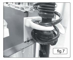
▲ DANGER Stop compressing the spring before the coil windings touch/bind.
