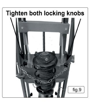
6.2.1. Offer the new strut spring up to the compressor's yokes and fit it in the same position as that of the old spring.
